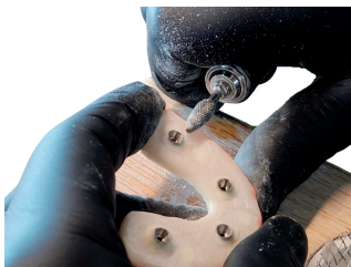
Remove Excess Material
